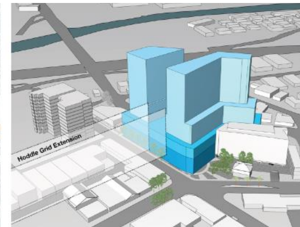
An alignment with the grid and serviceway splits the LEP envelope into two slenderly proportioned forms.
